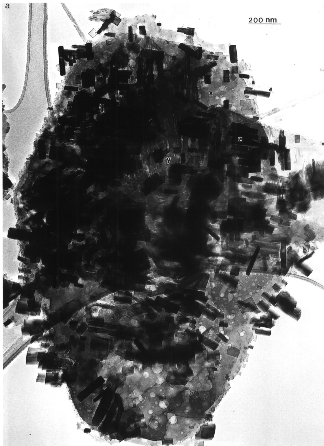
FIG. 8. Transmission electron micrographs from the VPO activated catalyst: (a) bright field micrograph showing disordered (VO)_2P_2O_7 (x), \delta - VOPO_4 (y) platelets and rectangular crystallites of (VO)_2P_2O_7 (z); (b) an axial HREM image from the [021] projection of (VO)_2P_2O_7 ; (c) an axial HREM image from the [100] projection of (VO)_2P_2O_7 ; (d) schematic diagram showing the morphology of the rectangular (VO)_2P_2O_7 crystallites.
